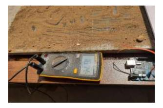
After installing the dust cleaning system, the solar panel performance improved considerably. When the LDR sensor detects a decline in light intensity, the cleaning mechanism starts the wiper, which removes the dust layer from the panel surface. As a result, the solar panels regain efficiency by enabling more sunlight to enter and be converted into power. The obtained output voltage after cleaning is 19.99V.
